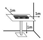
For best operation, the receiver should be at least 1m above the ground and 1m away from a wall or metal surface to minimise reflections. The transmitter should also be at least 1m away from a wall or metal surface to minimise reflections. The transmitter should also be at least 1m away from the receiver. Keep antennas away from noise source such as motors, automobiles, neon light and large metal objects.
